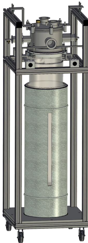
Fahrbares Gestell aus Aluminium Profilrohr Mobile frame made of aluminum profile tube
