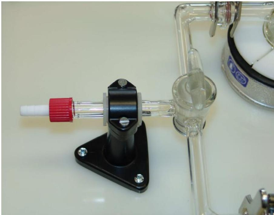
6. Produce a connection to the vacuum pump.
