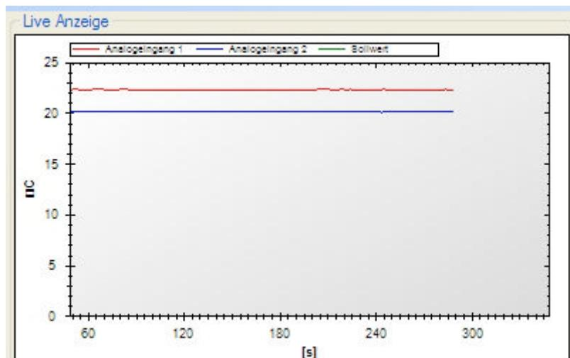
The live display graphically indicates the current temperature values of temperature 1 (Kaltgas sensor), temperature 2 (temperature sensor) and the target value.
