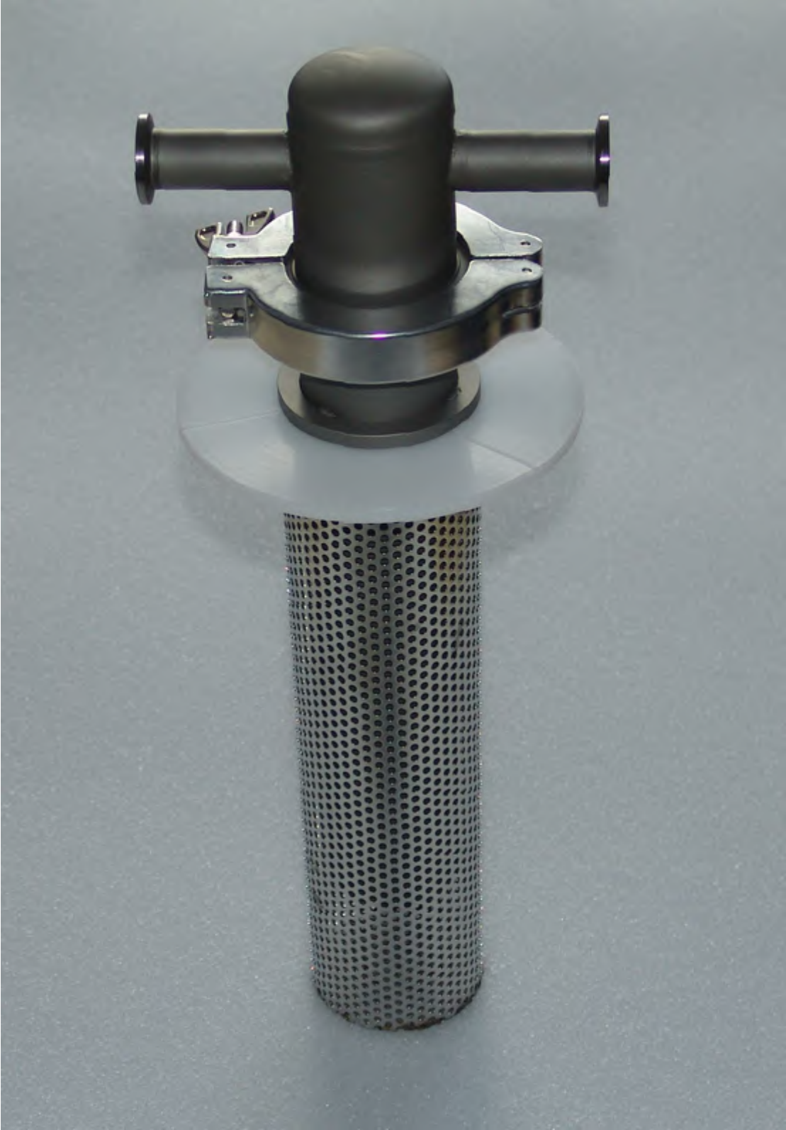
cold trap S54V-KW16-Z with CO2 wire basket
