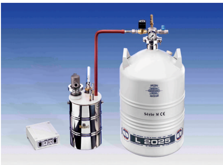
Automatic LN2 - level control with a stainless steel cold trap S 54V-K16-Z, Dewar flask, lid, gas outlet tube and LN2 store vessel with 25 litre. Art.No. 2750-25
