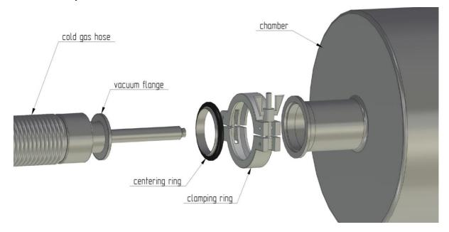
2. Using the corrugated hose to connect the cold gas line to the vacuum pump and using the vacuum pump, evacuate the cold gas line for at least 20 minutes before the start of the work.
