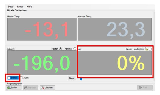
Here, care must be taken that before any adjustments are made to the JET or the set point temperature, the hook at power is removed, in order to avoid an unwanted start of the system. If the hook is removed, the settings can be changed without risk to the user and the system. If the settings have been changed, the hook must be set again to start the system.
