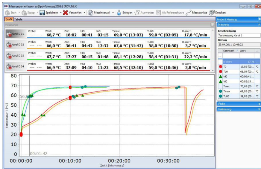
Measurement data acquisition with nlk 3
